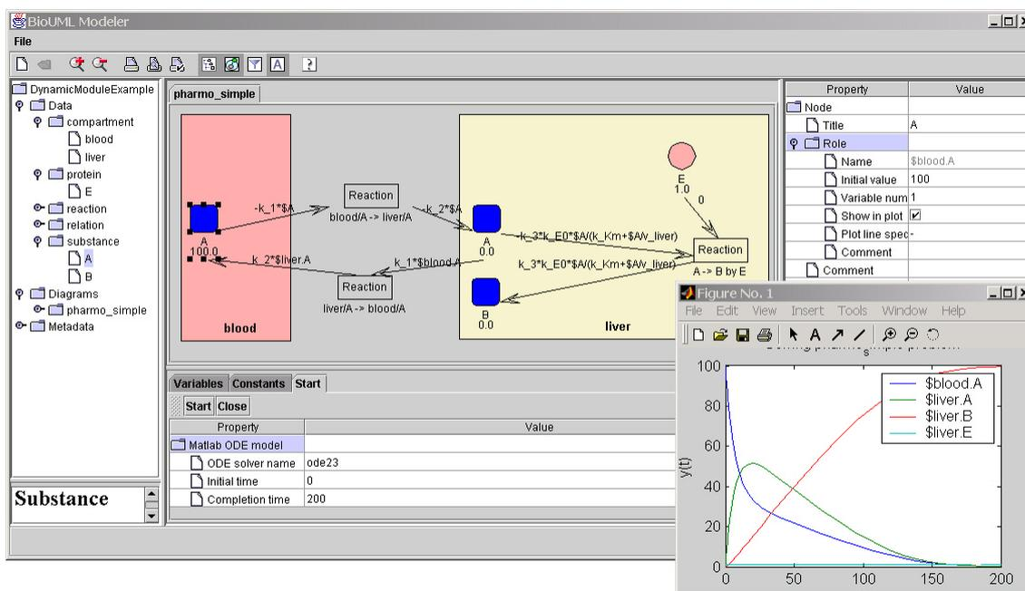
**Fig. 3.** BioUML modeler graphic user interface. Strings above arrows are right sides of differential equations associated with graph edges; numbers – are initial values of corresponding variables associated with graph nodes. Bottom right – result of model simulation using MATLAB.
