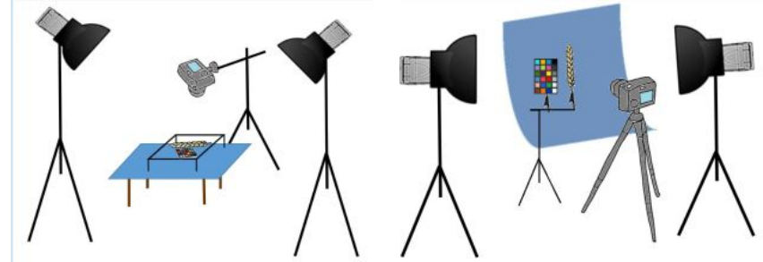
Fig 2: Scheme of photoing: ( left - on table, right - on pin )
